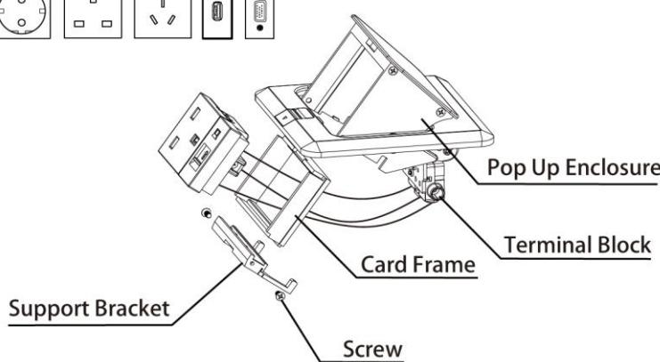
\*The unit is supplied with Type 45 (F) module card frame. The other type module card frames are available on request
